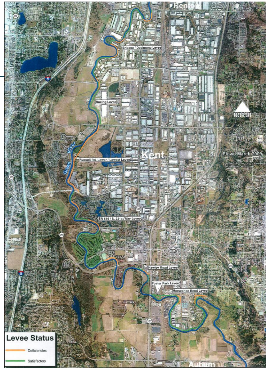
Levee Deficiencies May 2012
