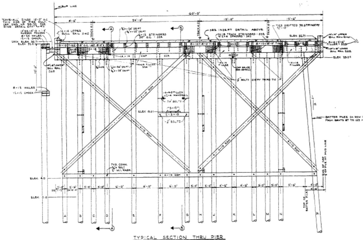
Figure 1 – Berth 410 typical pier section
