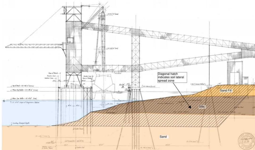
**Figure 6 – Berth 501 dock section indicating zone of soil lateral spreading**
