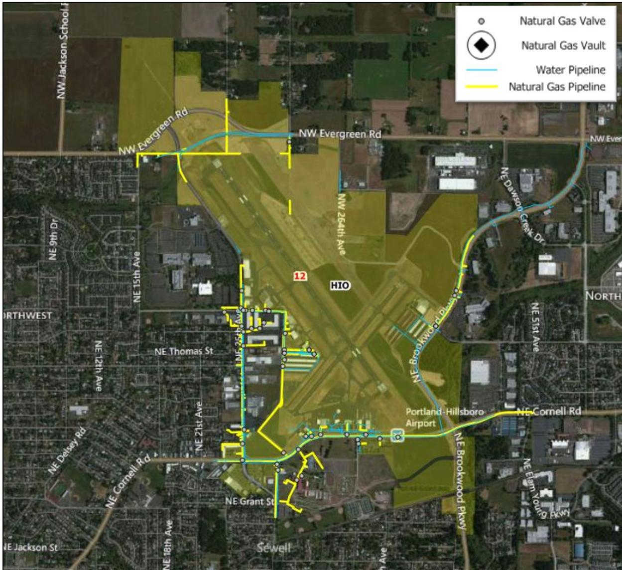
**Figure 15: Onsite Natural Gas and Water Pipelines at the Hillsboro Airport (Sources: Port of Portland)**
