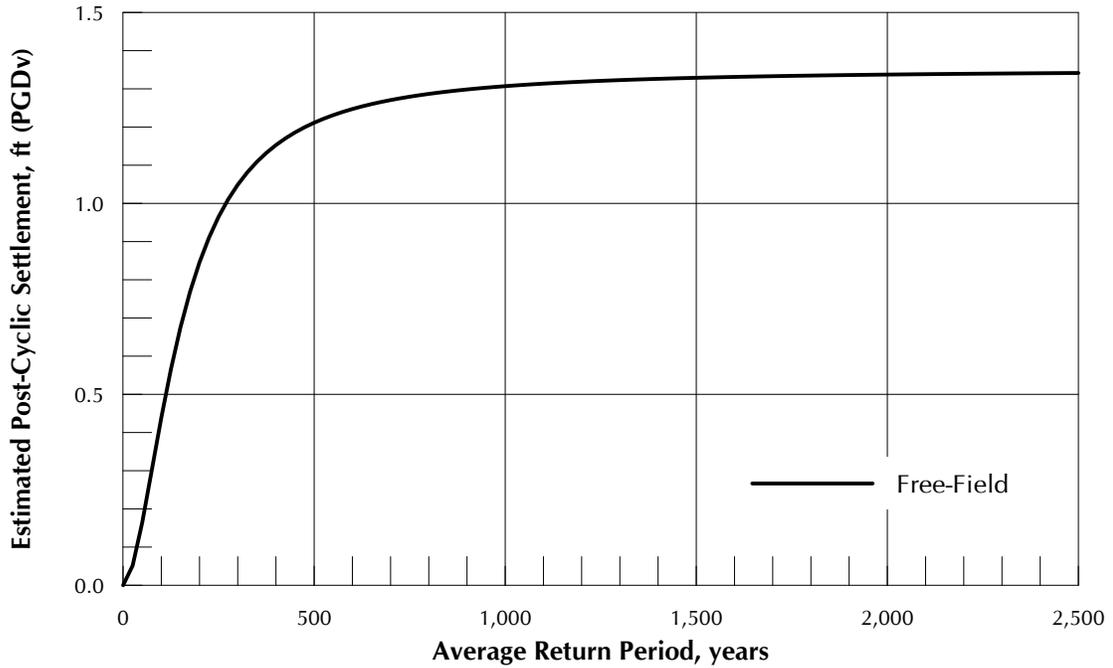
Note: Additional settlement of continuous perimeter footings is not anticipated. Additional settlement of isolated column footings is not anticipated at the 72-yr hazard level. To estimate the additional settlement of isolated column footings at return periods greater than 72 yrs, add 0.5 in. to the free-field settlement.
