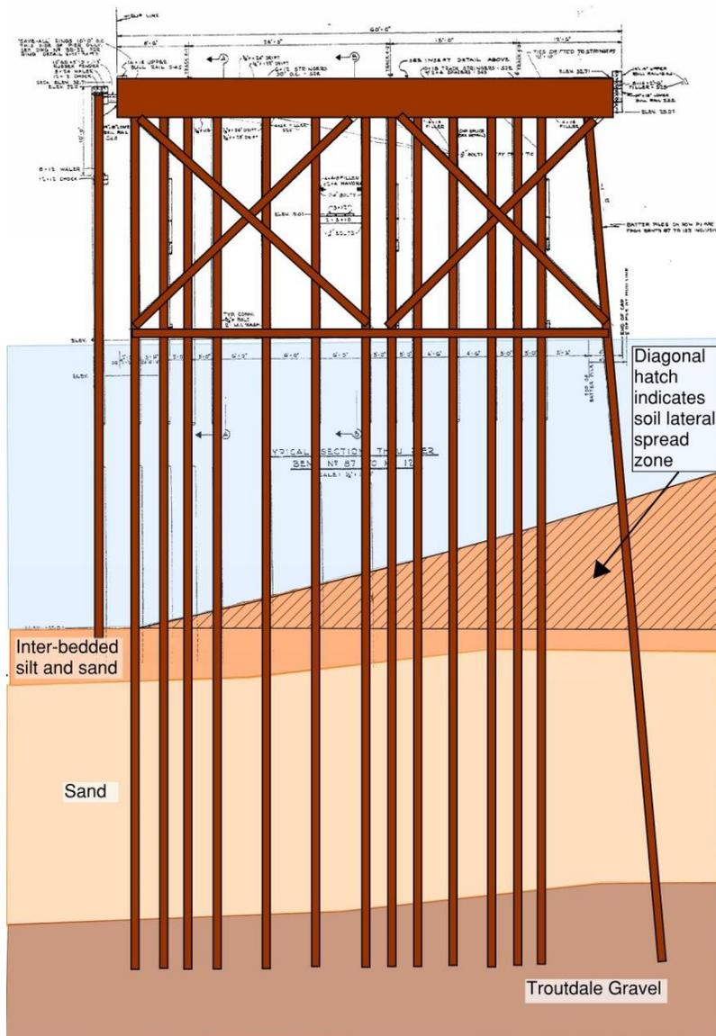
**Figure 2 – Berth 410 typical pier section indicating zone of soil lateral spreading**
