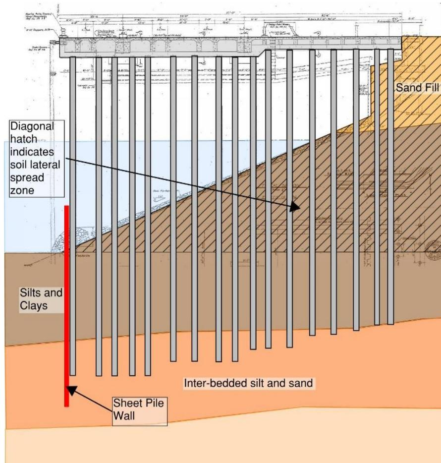
Figure 4 – Berth 411 typical wharf section indicating zone of soil lateral spreading
