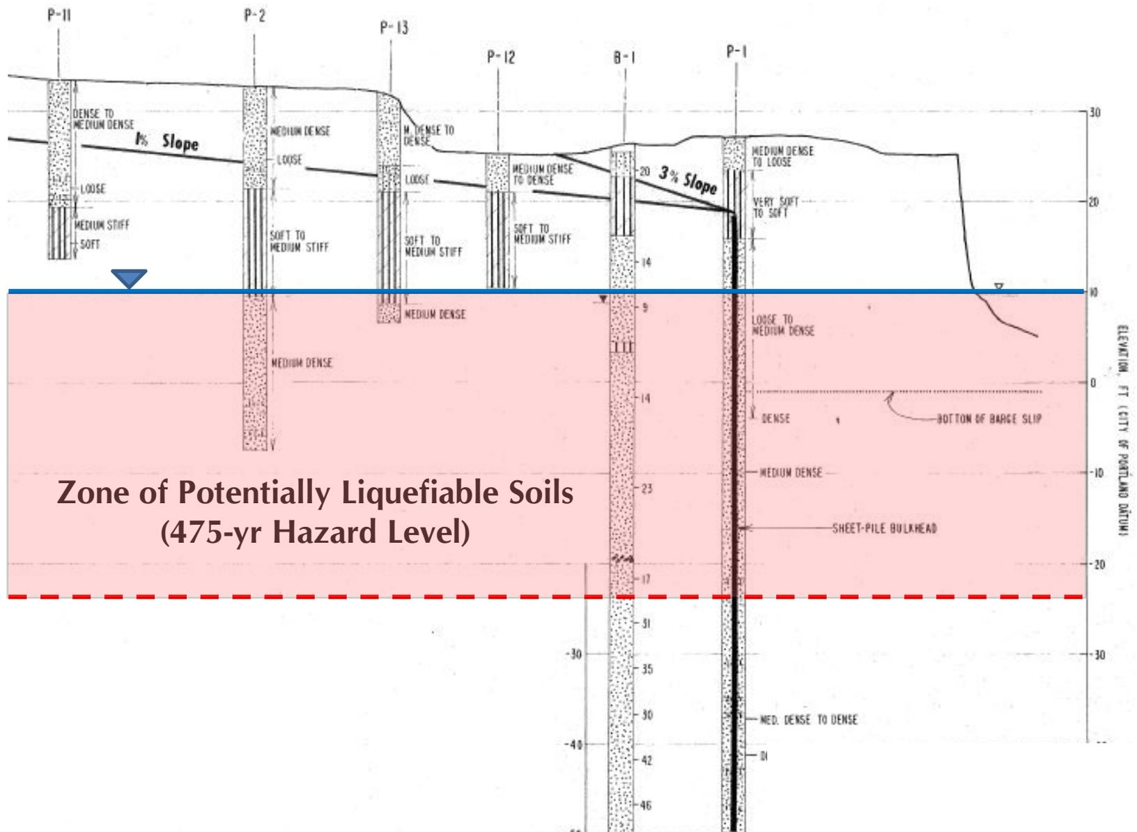
**Zone of Potentially Liquefiable Soils
