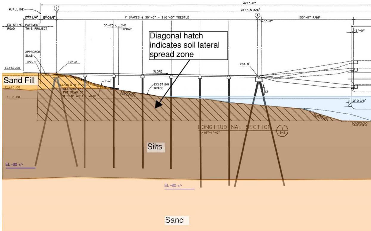
**Figure 11 – Berth 601 trestle longitudinal section indicating zone of soil lateral spreading**
