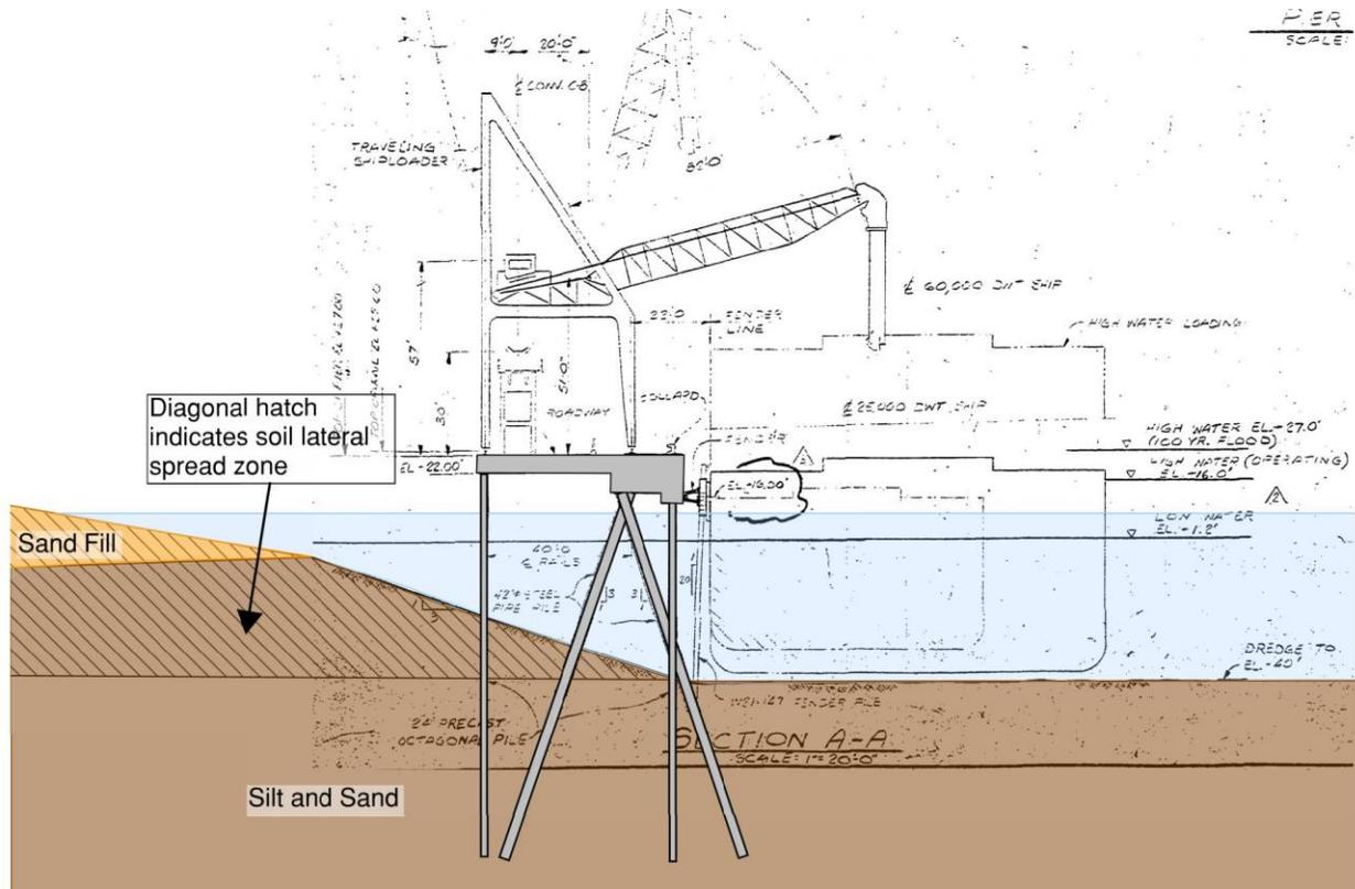
**Figure 8 – Berth 503 dock section indicating zone of soil lateral spreading**
