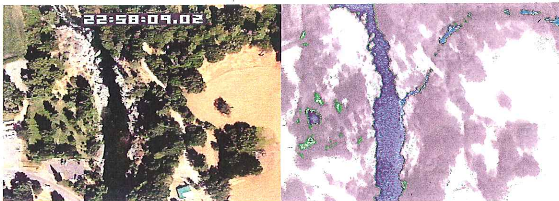
Figure I-3 - Day TV/FLIR Image pair showing the confluence of the Applegate River (20.6 deg C) and Thompson Creek (18.4 deg C). The Applegate River flows from the top to bottom of the image and Thompson Creek flows in from the right side of the image. The thermal contrast between Thompson Creek and the surrounding terrain makes it easy to detect in the thermal image while it is not so apparent in the day TV image. ( frame app0648 ).
