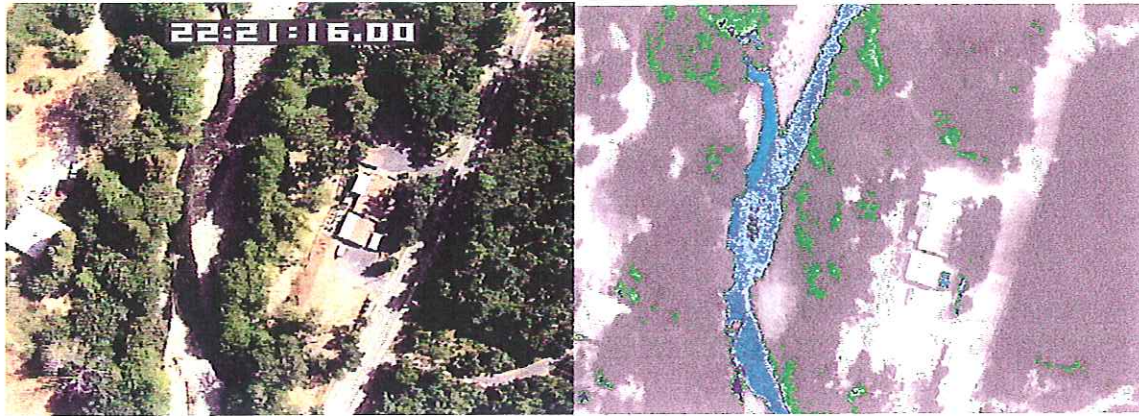
Figure I-9 - Day TV/FLIR image confluence of East Fork and West Fork Williams Creek. Williams Creek flows from the top to bottom of the image. The East Fork flows in from the left side of the image. A gravel bar at the confluence is detectable in both the day TV and thermal image. ( frame wil0413 ).
