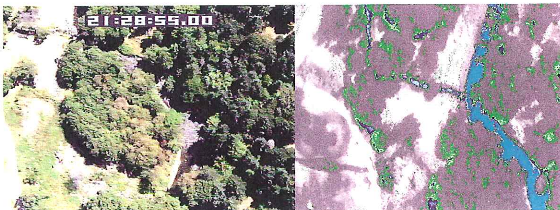
Figure I-4 - Day TV/FLIR Image pair showing the confluence of the Little Applegate River (17.6 deg C) and Sterling Creek (19.9 deg C). The Little Applegate River flows from the top to the bottom of the image. The day TV and thermal image frames were collected simultaneously from two different instruments and there is often a slight (but inconsistent) time shift between the two images. This is evident in this image pair where Sterling Creek is evident in the middle of the thermal image, but it near the top of the day TV image. ( frame: la0202 )
