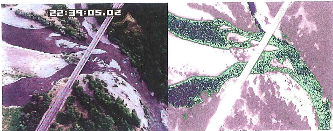
Figure I-2 - Day TV/FLIR Image Pair showing the confluence of the Applegate River (23.0 deg C) and Slate Creek (21.9 deg C). Tributaries are often visible in the thermal image. When the tributaries are identified, the surface water temperature is sampled using the same methods used to sample the mainstem. Tributaries and other off channel features are identified from base maps, the day video, and other features such as the bridge. ( frame app0076 ).
