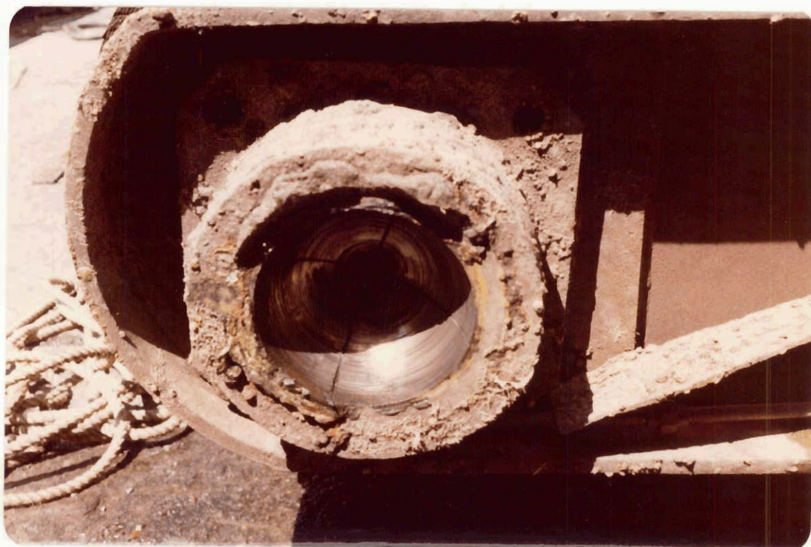
Frame ② 4 May 82 Pintle Bushing for Rt. Leaf - 3 bolts Sheared
